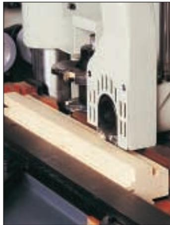
The groove spindle works precisely to within a fraction of a millimeter, i.e. the groove for the window sill and nosing. Important for renovation work on old buildings: various groove depths.
