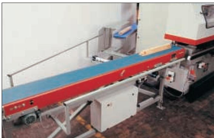
Return roller conveyor: The workpieces are returned to the operator in the correct position. This saves the cost of an operator at the machine outfeed.
