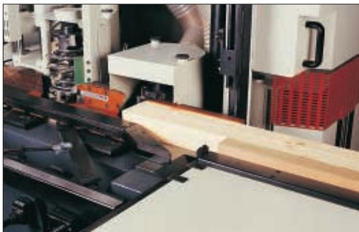
The special guide fence enables machining of parts of random width up to 100 mm. Without any manual adjustment you can machine for example a mullion of 110 mm width and a glazing bar of 50 mm width, one after the other.
