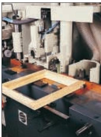
Stormproofing with a climb-cutting spindle. This turns your Weinig Unicontrol 6 into an automatic stormproofing machine. Controlled feed rollers reduce throughfeed time.
