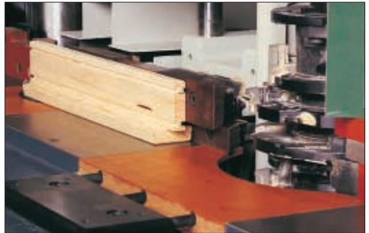
Extremely close distance between feed rollers. The fence is controlled. Thus very short and narrow glazing bars can be produced.
